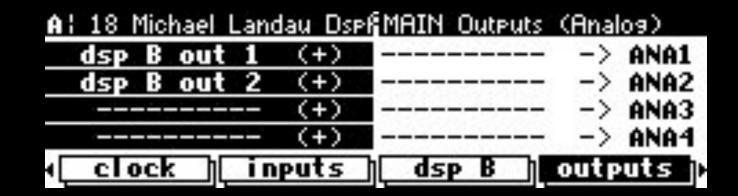
And out we go, connecting DSP B outputs to the unit analog outputs 1 & 2. So the overall signal flaw will be:
