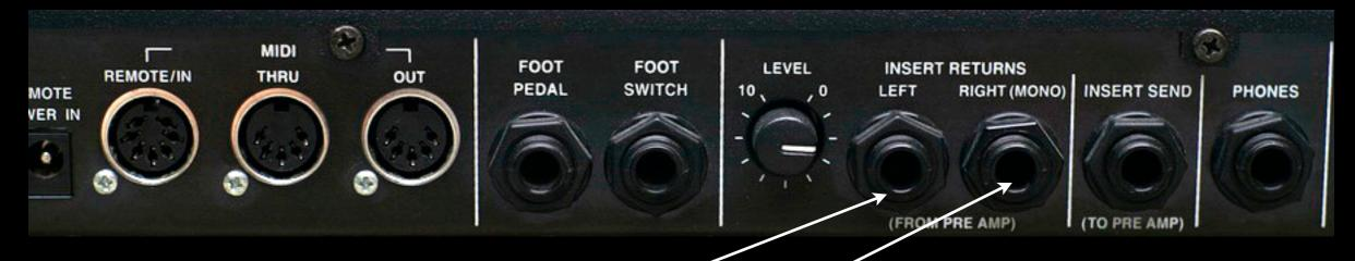
Connect your preamp or mixer/DAW AUX Send to the RIGHT INSERT RETURN to process MONO signals. Use both INSERT RETURNS for STEREO signals. Set the LEVEL at about 4 (don't mind the picture for this) and check the front panel Aux In LED. You may need to set the LEVEL to a different value, depending on your system signal strength.
